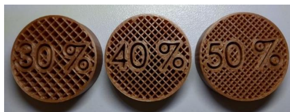
Figure 2. The percentage infilling effect on printed objects
